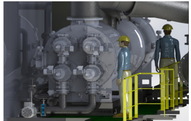
Figure 1: BWTS integration in Ship Model – Main Filters
